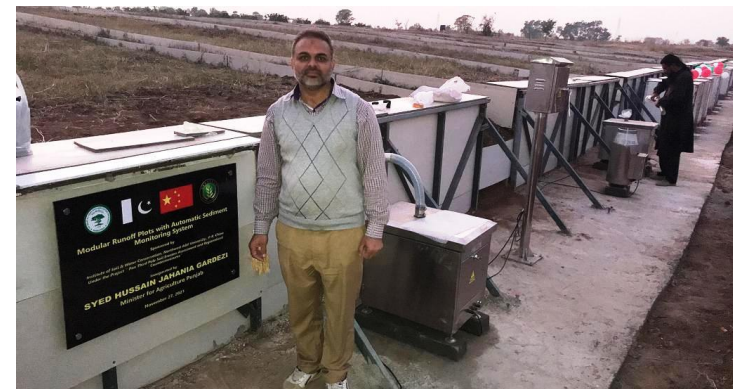
Figure: Automatic erosion assessment equipment
